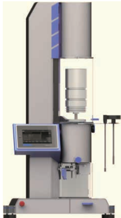
MeltFlow-Rheo 旗舰版，全自动砝码切换、加载、提升
